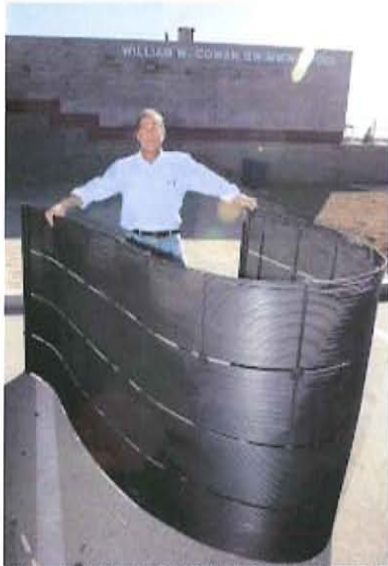
Solar Solutions President Gad A. Ronat holds up one of the solar panels that will be installed later this month at William W. Cowan aquatic center in the Lower Valley. It is one of nine pools that will have solar panels installed to heat the pools with solar power and reduce the city's electric bill. (Photos by Ruben R. Ramirez / El Paso Times) City Hall.
